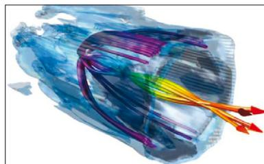
laser to send pulses of 800 nm wavelength light through the plasma. This generates a high-charge separation between the positively charged atomic nuclei from the electrons in the plasma to leave a wake of plasma waves in its path on which the electrons "surf" and pick up energy.
